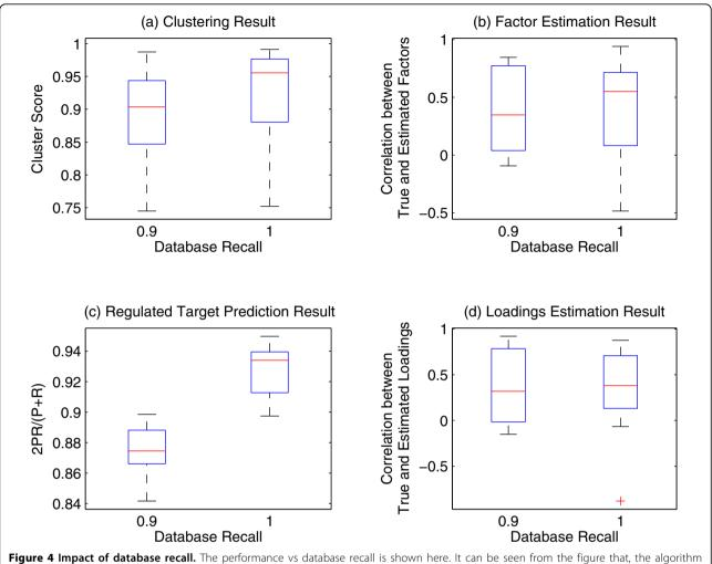
**Figure 4 Impact of database recall.** The performance vs database recall is shown here. It can be seen from the figure that, the algorithm performance deceases as noise increases. While the target prediction relies on the quality of database heavily (Fig.4-c), the clustering result is relatively robust against database quality (Fig.4-a).
